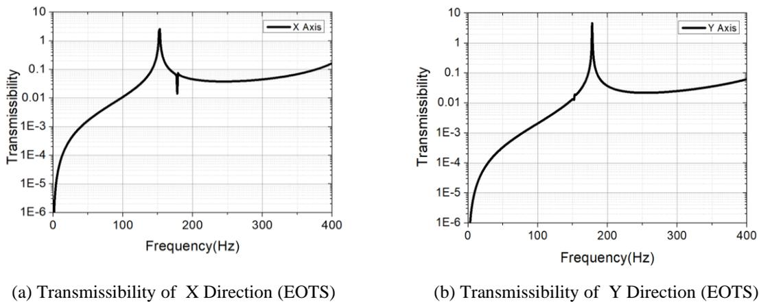
Figure.6 Transmissibility Graph (0~400Hz)
