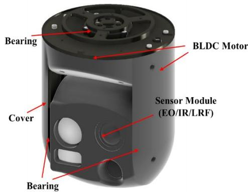
**Figure.1** Components of EOTS Structure
