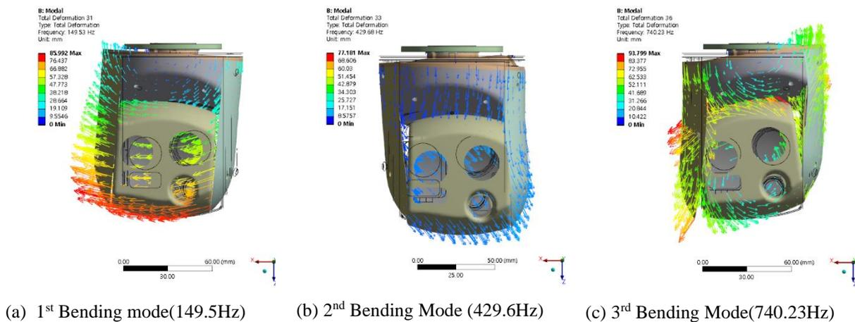
**Figure.3** Bending Mode Shape
