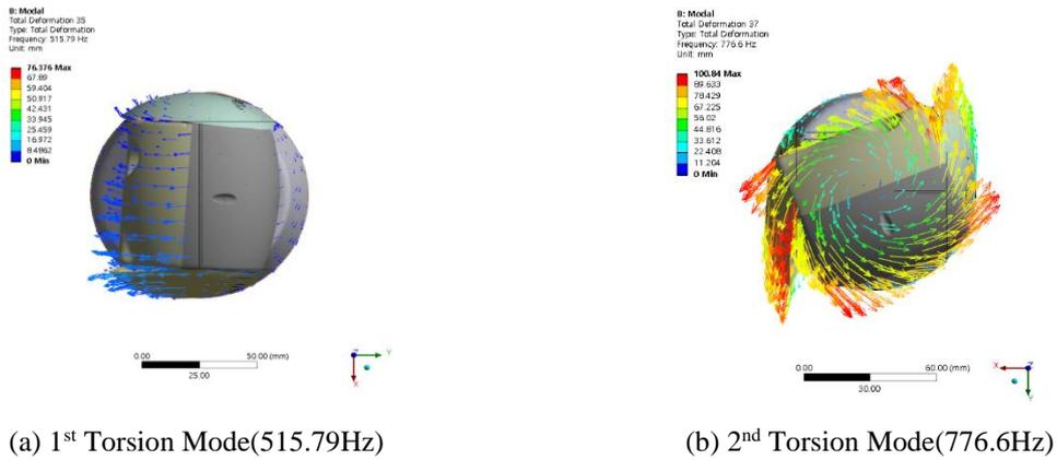
Figure.5 Torsion Mode Shape
