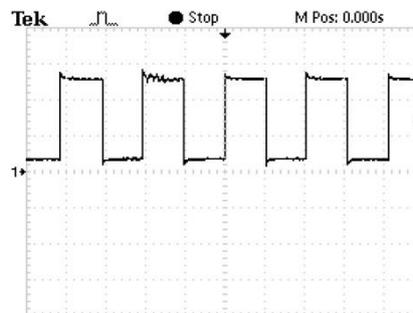
Fig.13. Gate signal for switch  $S_1$
