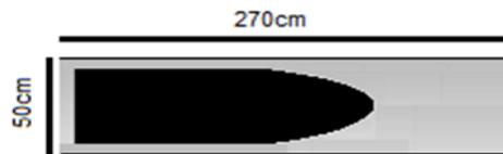
**Figure 1.** Projectile geometry, projectile barrel length: 270 cm, 50 cm in diameter
