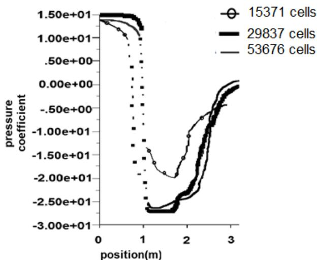
**Figure 4.** The discrepancy of pressure coefficient between the grid with the number of 29837 cells and the one with 53676 cells
