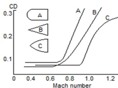
**Figure 3.** Rapid CD changes in the subsonic area for muzzle of different shapes [8]
