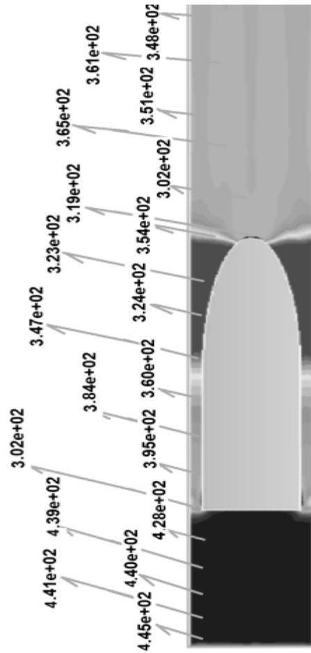
**Figure 13.** Temperature distribution inside the barrel of the weapon in Kelvin
