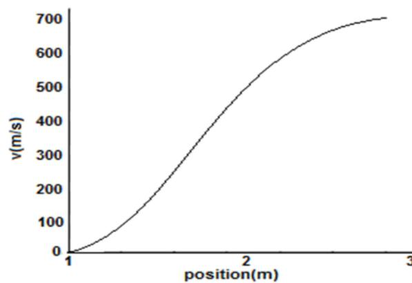
Figure 10. Velocity distribution over time inside the barrel of the weapon
