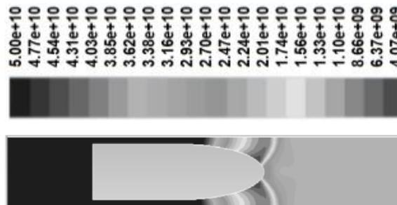
Figure 7. Static pressure distribution contour of the projectile
