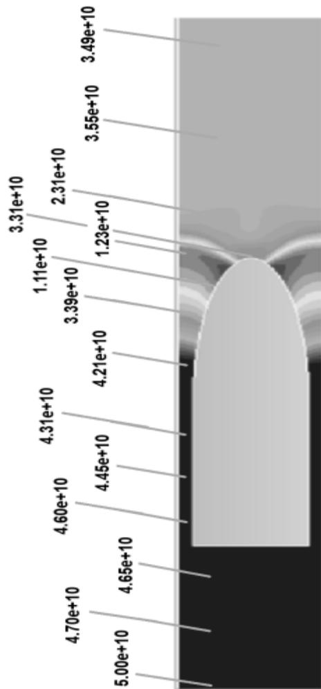
Figure 9. Static pressure distribution inside the barrel of the weapon by Pascals
