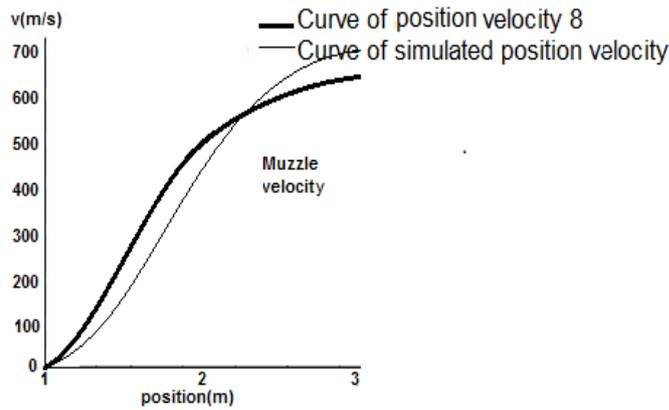
Figure 5. Validation of position velocity curves
