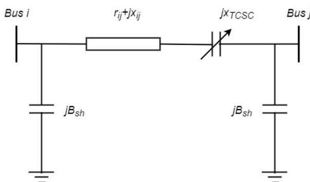
Figure 2.  $\pi$ -model representation of a branch with TCSC
