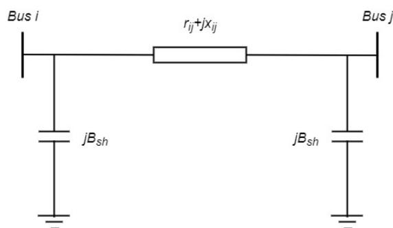
Figure 1.  $\pi$ -model of a line
