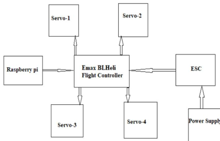
**Fig 11:** Block Diagram of drone**Create drone flight map plans**
