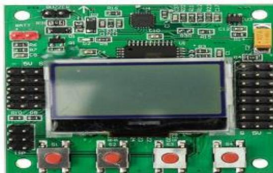
Fig 2: Flight Controller Board
