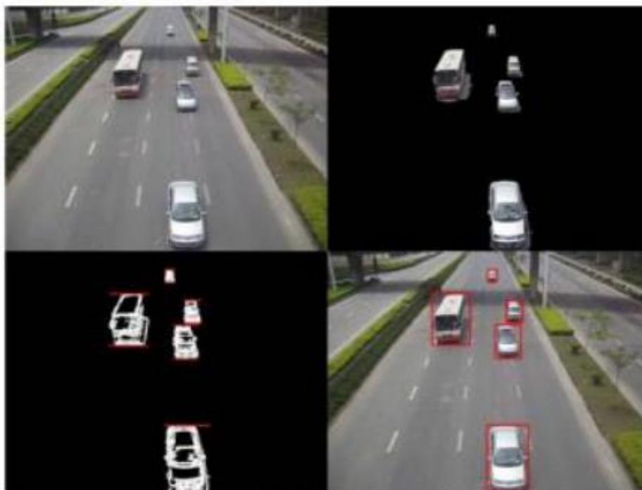
**Fig9:** Vehicles speed detection
