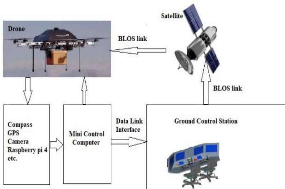
**Fig 12:** Block Diagram of Satellite Communication System**Drone Implementation**
