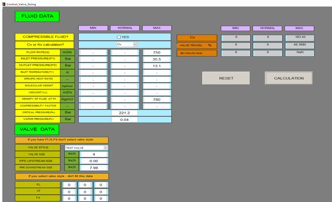
Figure 6-3: Calculating Cv using the neural network
