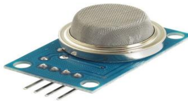
Figure 6 Gas Sensors for Air Quality
