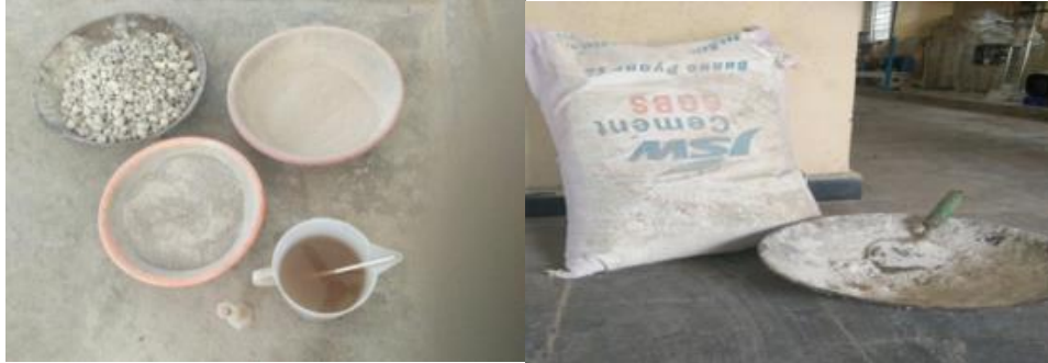
Figure 1: GGBS, Robo Sand, Coarse Aggregate, Activator Solution, GGBS
