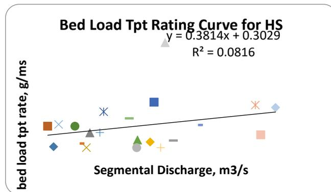
Fig. 6. Rating curve for bed load transport rate
