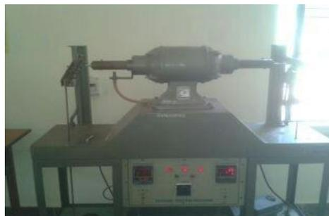
**Fig.6** Fatigue testing machine
