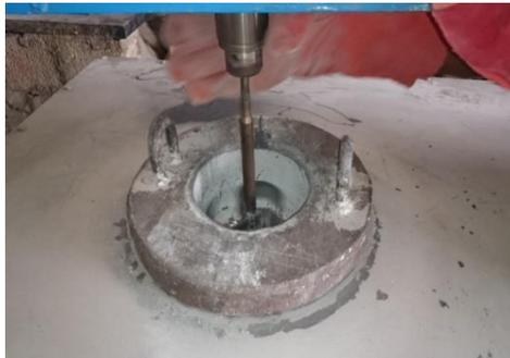
**Fig.2** Stir Casting furnace
