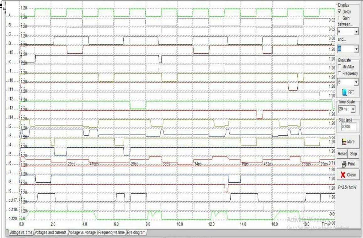
Fig10: Input and output waveform of 2bit comparator using 4:16 CMOS line decoder.
