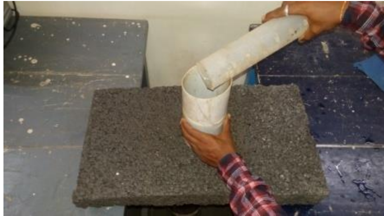
Fig 13: Rate of Infiltration
