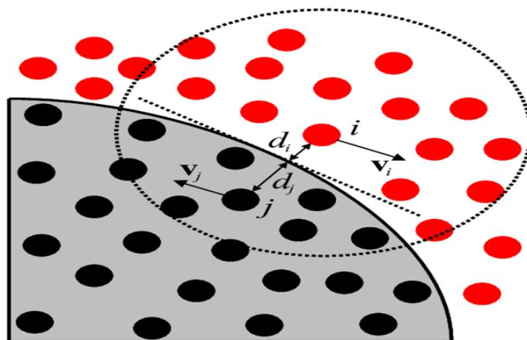
Figure 6: Analysis open boundary conditions in SPH simulations
