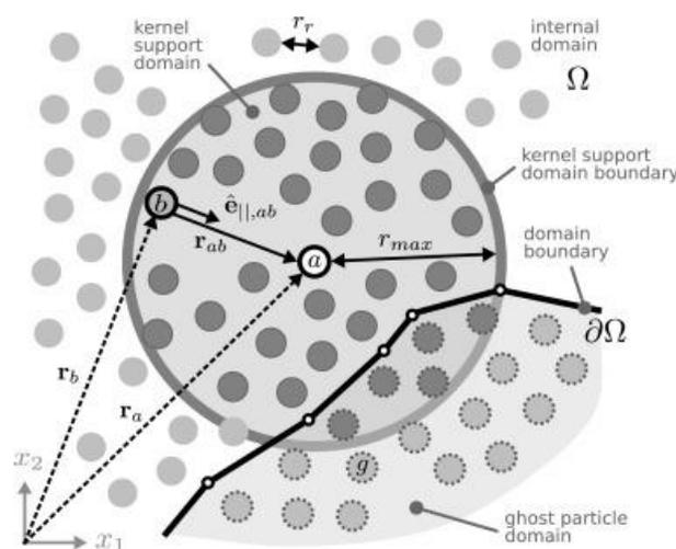
**Figure 5 : Smoothed Particle Hydrodynamics (SPH) simulations**
