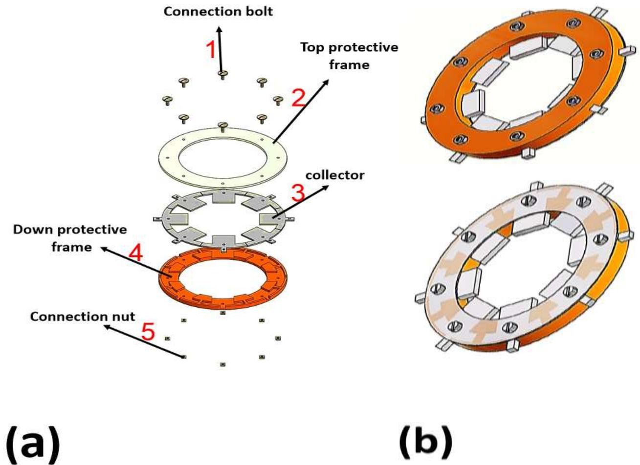
**Fig. 2** all the components of the collector
