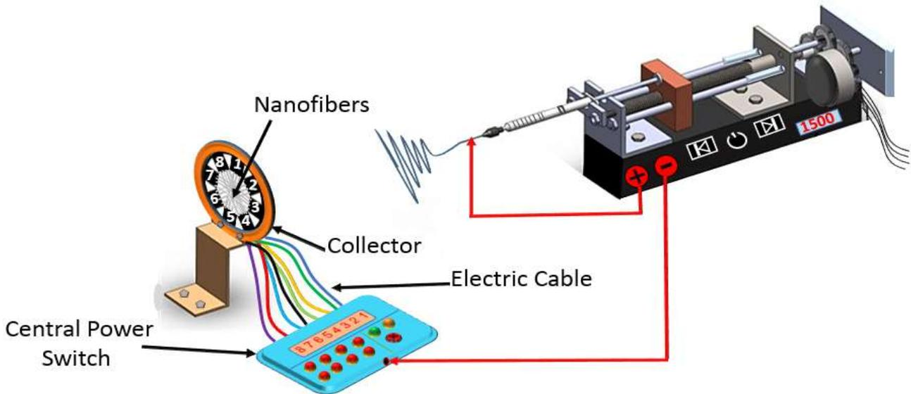
**Fig. 3** Overview of the electrospinning system and how the collector and central power control device are located.
