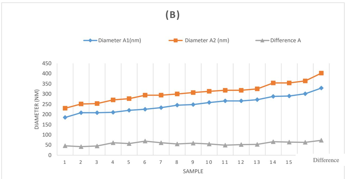
**Fig. 6** Comparison of diameter differences between two experimental samples (Unacceptable nanofibers).
