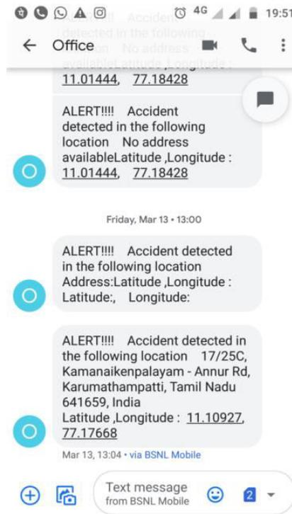
Figure 7(a).Alert message on Accident detection and location identification
