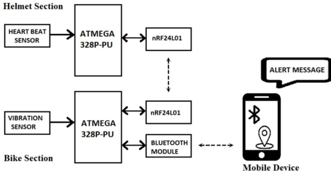
Figure 1. Interconnection of the proposed modules
