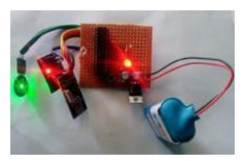
Figure 4. Hardware implementation of the proposed Helmet section
