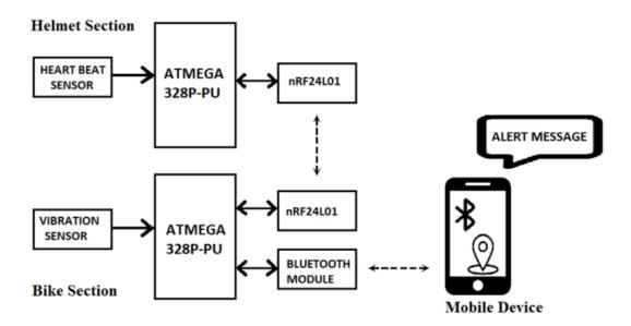
Figure 1.Interconnection of the proposed modules
