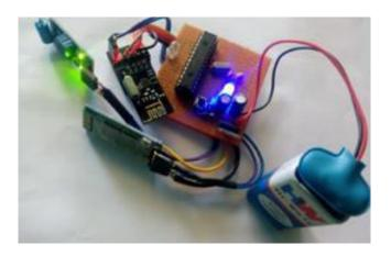
Figure 5. Hardware implementation of the proposed Bike section
